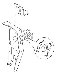
Pull the thread at the speed of 110mm/sed in the direction of arrow
