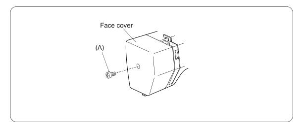
1. Remove the face cover by removing the setscrew (A).
